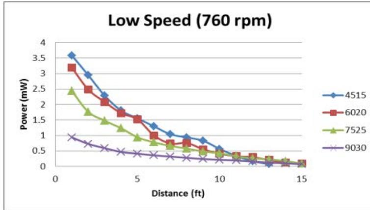
a) Data collected with the fan running at low speed (760 rpm).
