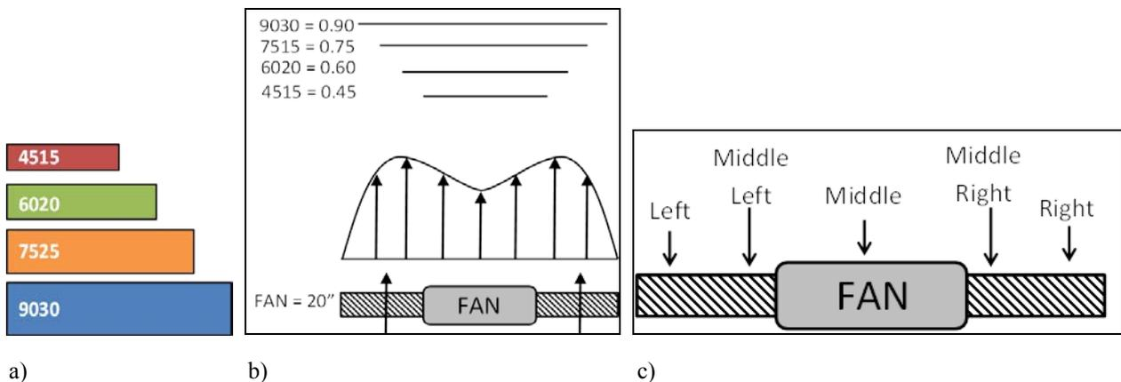
Figure 3: a) A proportional representation of the size of each set of turbine blades; b) A velocity profile of the flow from a fan and the ratios of the diameters of the four kinds of turbine blades tested to the diameter of the fan that was used during experiments; and c) The five locations in the cross section of the flow from the fan where the air speed was sampled using an anemometer. Sampling was done at many flow cross sections.
