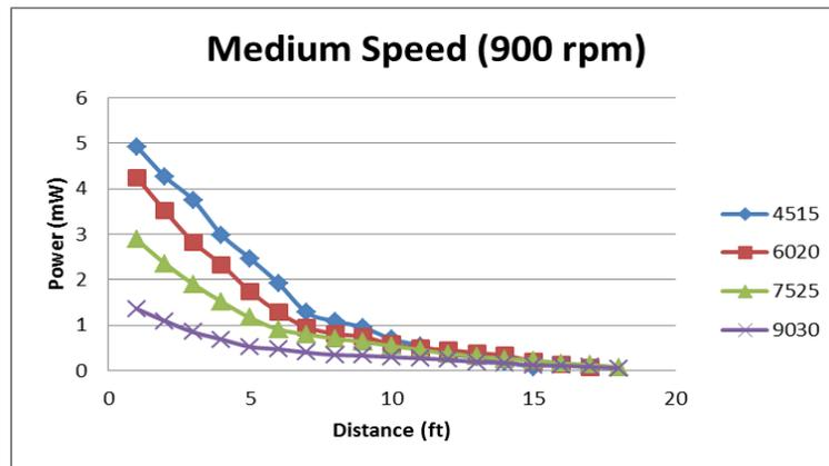
b) Data collected with the fan running at medium speed (900 rpm).
