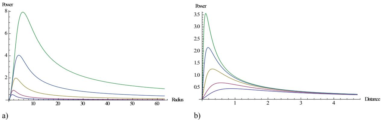
Figure 2: A series of curves, plotted from Equation (9), showing how power produced by a turbine varies a) with the radius of the turbine blade, at fixed distances from the turbine; and b) with distance between the fan and the turbine, at fixed blade radii. In both plots, a fixed rate of mass flow is assumed to issue from the fan.
