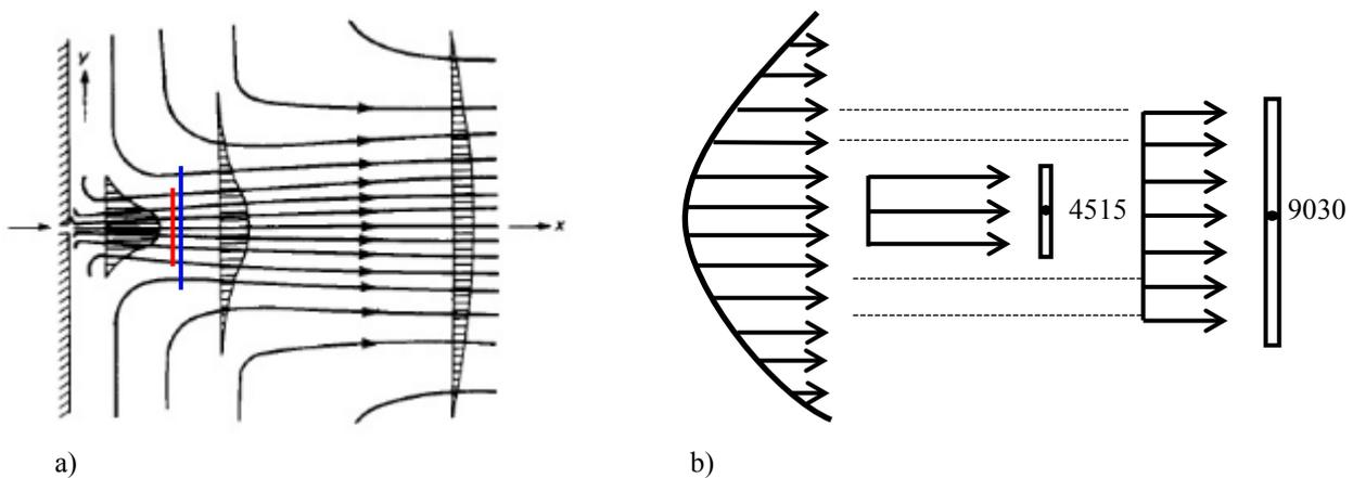
Figure 1: a) A series of two-dimensional velocity profiles (plotted from Equation (6)) of a laminar free jet superimposed onto a pattern of streamlines for that flow [7][10]; b) A graphical representation of a non-uniform velocity distribution and the averaged air speeds on the faces of two turbine blades of different radii. Turbines 4515 and 9030 are shown here. These turbines are described below.
