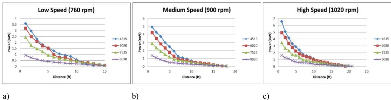
Figure 4: Power produced by four different turbines versus distance between the fan and the turbine under three different conditions: a) low fan speed (760 rpm); b) medium fan speed (900 rpm); and c) high fan speed (1020 rpm).
